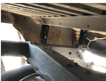
Rear tub lift blocks
