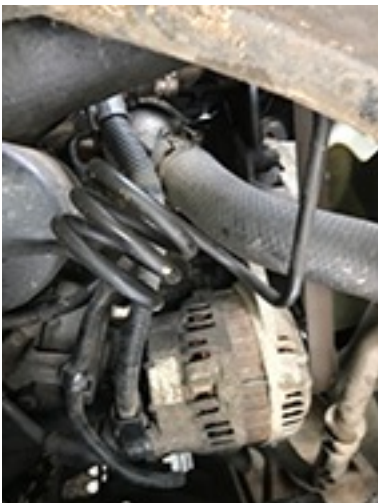
This is the front brake line note the coil which will accommodate a 4" lift
