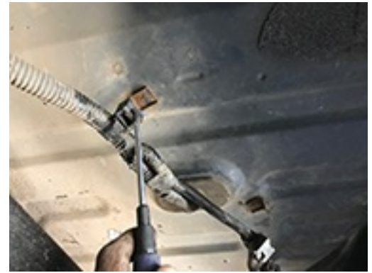
One of the cables on the tub that need to be unclipped
